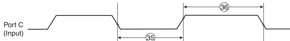
Figure 48. Port C Interrupt Detection Timing
